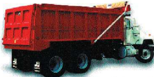
DynaHauler/MLWC, a light-weight, cross-memberless steel body that features newly designed formed bottom rails.
